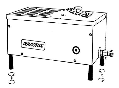
Distillers operate properly when condenser coil has a constant downhill slope. To level distiller on uneven surfaces, unscrew one or two legs at opposite corners to achieve proper height and stability.
