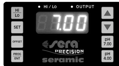
**pH 7** Rinse the electrode with distilled water and immerse it into the green sera test solution pH 7.0. Wait for at least 60 seconds. Press the keys
