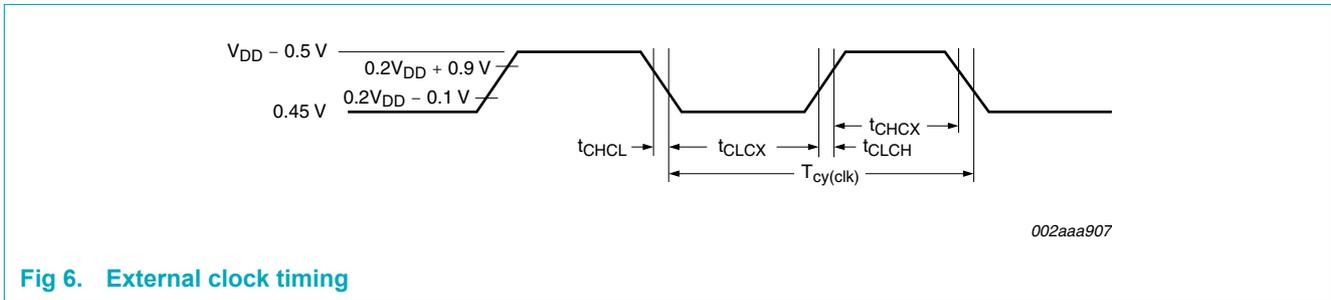
Fig 6. External clock timing
