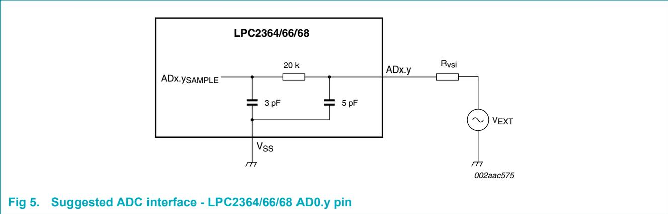
Fig 5. Suggested ADC interface - LPC2364/66/68 AD0.y pin
