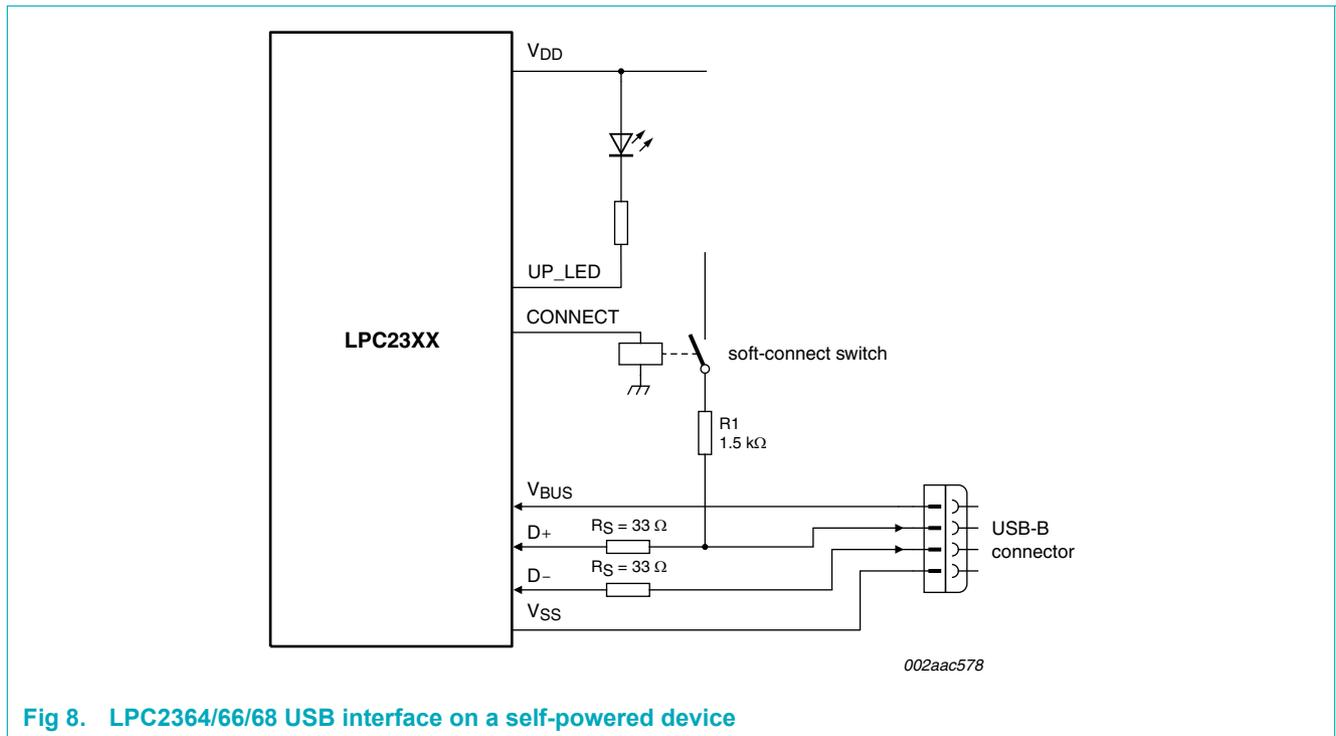
Fig 8. LPC2364/66/68 USB interface on a self-powered device
