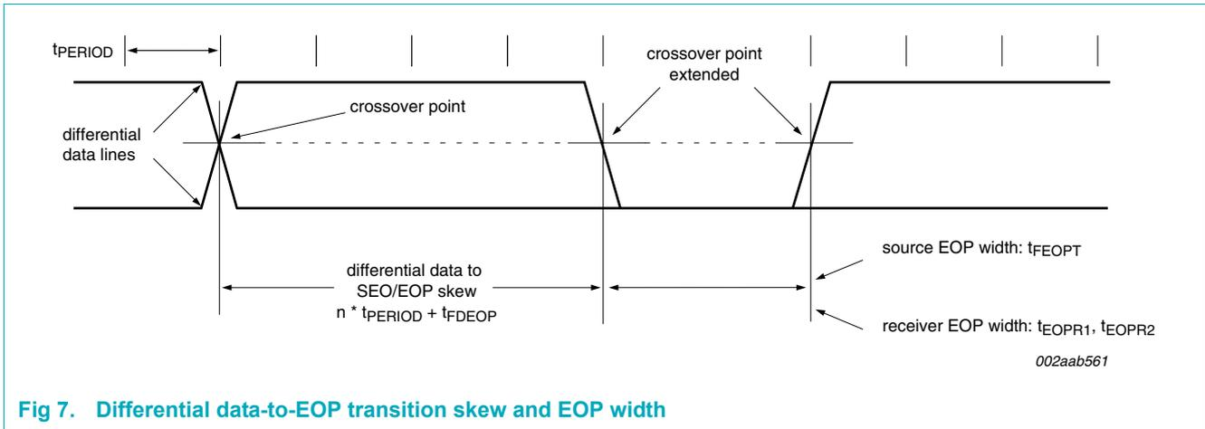
Fig 7. Differential data-to-EOP transition skew and EOP width
