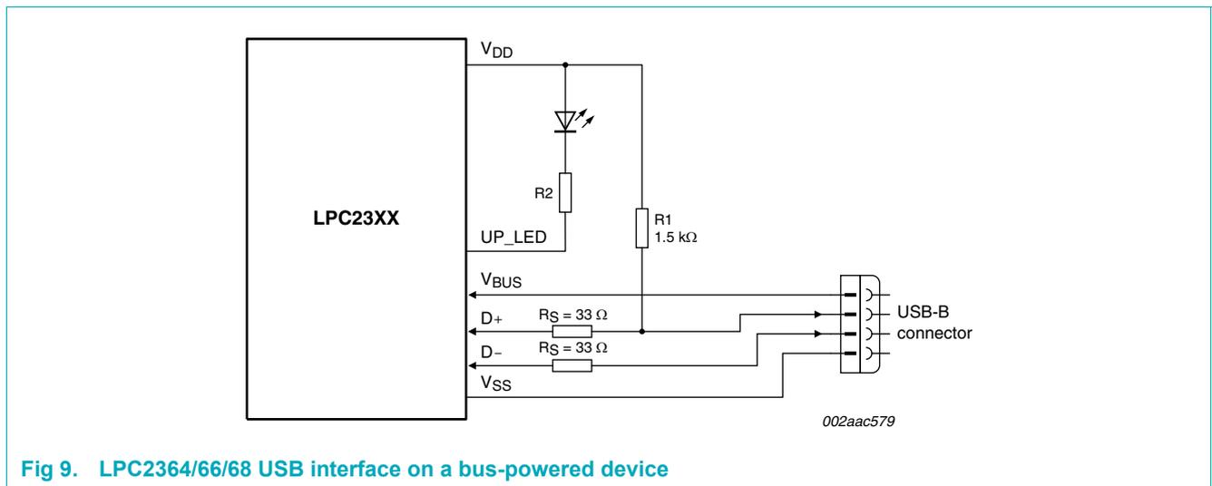
Fig 9. LPC2364/66/68 USB interface on a bus-powered device
